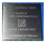
Operating frequency bands and related max radio-frequency power transmitted: LTE: Bands B1, B3, B5, B7, B8, B20, B28, B34, B38, B40, B41:25dBm
