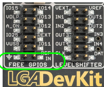
Figure 16: External reference supply and pin header for free level shifter
