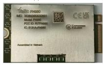
Operating frequency bands and related max radio-frequency power transmitted: 3G: Band I, Band III and Band VIII: 25,7 dBm
