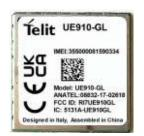
Operating frequency bands and related max radio-frequency power transmitted: E-GSM/GPRS 900: 33.5 dBm, EDGE 900: 28 dBm
