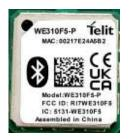
Max radio-frequency power transmitted: 18.94 dBm (EIRP)
