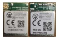
Operating RF frequency range: 2400MHz to 2483.5MHz
