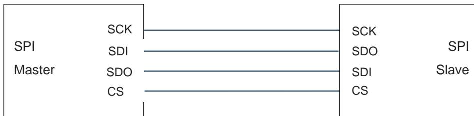
Figure 6-1: SPI Master-Slave Connection
